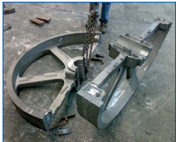
Bursting of pulley for optimal fracture pattern
